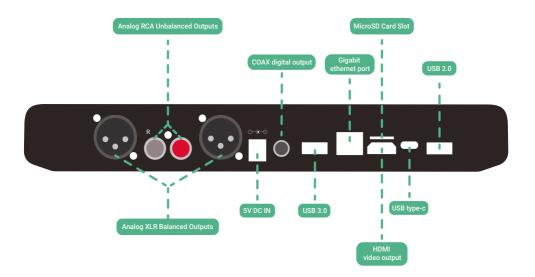
**ANALOG XLR BALANCED OUTPUTS:** XLR Balanced Output connection will output 4V RMS allowing you to run longer lengths of wire without picking up interference. If you own an amplifier with XLR inputs, this connection gives you a cleaner audio signal. Suggested connection to achieve best performances from Primo's integrated high resolution DAC.
